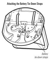
Route the power cable from the mount DOWN through the center hole of the base. Route the transducer jump cable UP through the base and mount.
